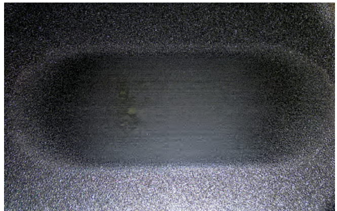
New Eclipse after 700,000 cycles. The coating has been polished, and shows some wear, but continues to perform.
