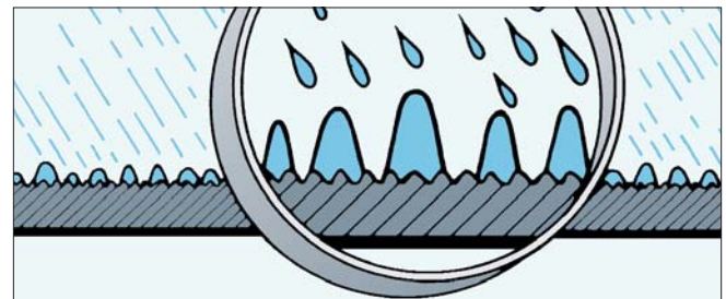
2. Then, the most important part: White-hot particles of a special stainless steel (an alloy patented by Whitford) are sprayed onto the roughened surface.
