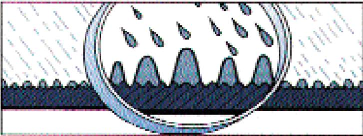
**2.** Then, the most important part: white-hot particles of a special stainless steel (Whitford's patented alloy) are sprayed onto the roughened surface.
