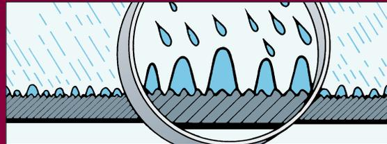
2. White-hot particles of a special stainless steel are sprayed onto the surface, cooling and hardening.
