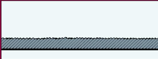
1. First, the surface of the pan is blasted to roughen it, so that other elements in Excalibur adhere better.
