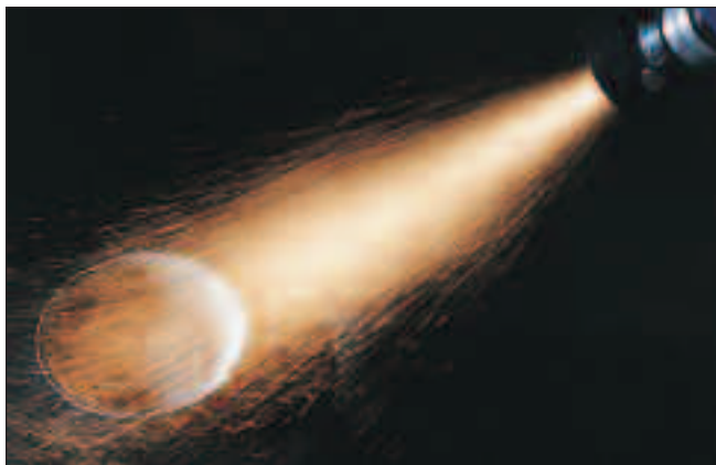
The secret of Excalibur's durability: a patented stainless-steel alloy that forms a hard matrix into which three coats of tough nonstick are sprayed.
