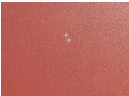
"Fish eyes", small holes caused by contaminants (such as fingerprints) on the surface.
