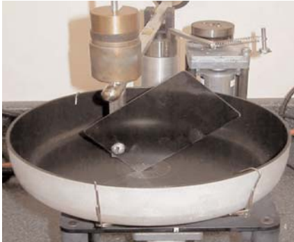
Whitford's Knife Cut and Scrape Test: a fast, reliable way to measure the wear resistance of a coating.
