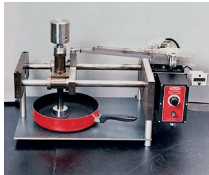
The Reciprocating Abrasion Test replicates marring from scouring, stirring spoons, etc.
