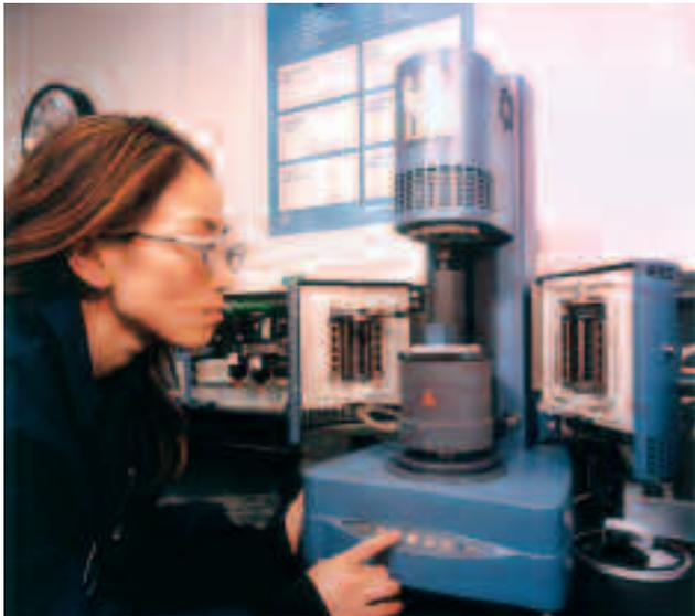
**TA Instruments R200 Rheometer:** Measures the flow and deformation of component materials in a coating formula, key to film formation, curing and aging. Understanding and analyzing the rheology of a coating is crucial for maximizing its performance.
