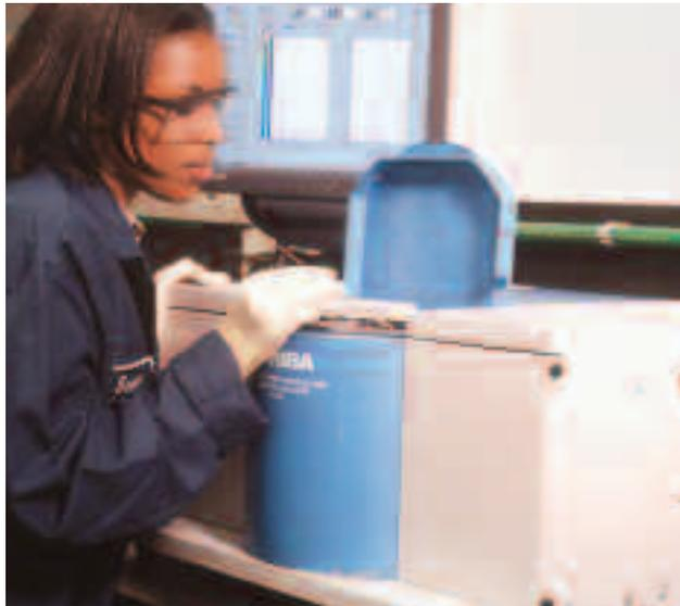
**Horiba LA-910 Particle Size Analyzer:** Measures the precise size of particles. This is crucial to quality control since particle size can affect stability, chemical reactivity, opacity, flowability and material strength. This equipment provides an analysis of sizes in 20 seconds.
