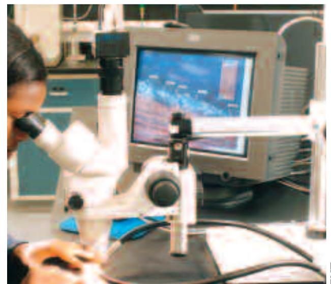
**Nikon Zoom Stereomicroscope:** One of its primary uses is to measure the dry-film thickness of applied coatings by providing a clear view of a tiny cross-section placed under the microscope. It can also detect improper inter-coat adhesion, a cause of coating failure.
