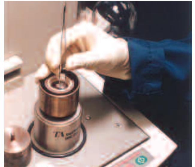
**Differential Scanning Calorimeter:** Determines the flow of heat into or out of a material. This is important in identifying melting points and phase transitions as well as glass-transition temperatures, which in turn provide information about stability, identity, purity and quality.
