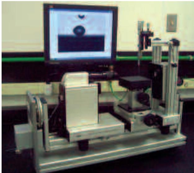
**Drop Shape Analyzer DSA10:** Just as rain beads up on a freshly waxed car, a drop of liquid should bead up on a coated surface. Measuring the angle of the bead against the surface provides the contact angle. The higher the angle, the better the release.
