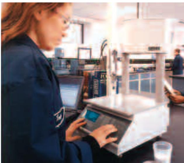
**Dynisco Melt-Flow Index:** Measurement of polymer flow indicates whether it will flow out properly when applied. Increased or decreased flow rate can indicate incorrect molecular weight, degradation, etc., which can mean loss of strength, impact and chemical resistance.
