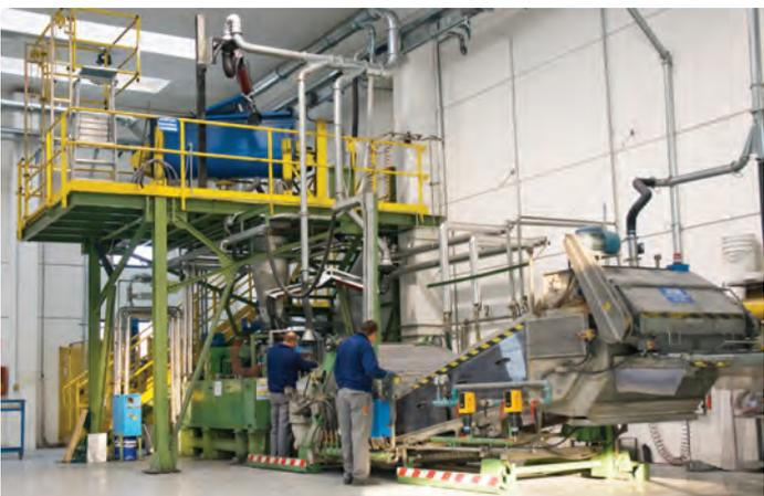
The new facility for housing the powder extruder and cooling belt.
